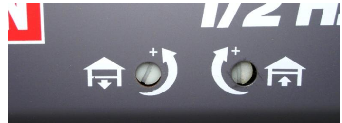
Up and down travel limit adjustments
