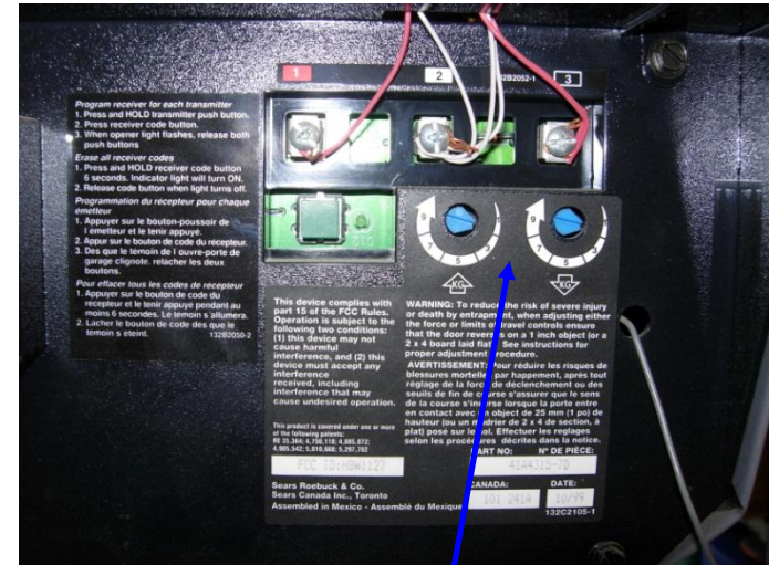
Up and down safety reversal force setting adjustments
