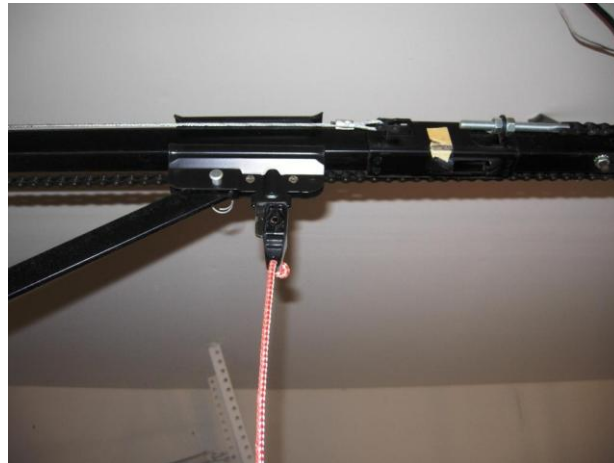
Door can move freely when lever is pointing down
